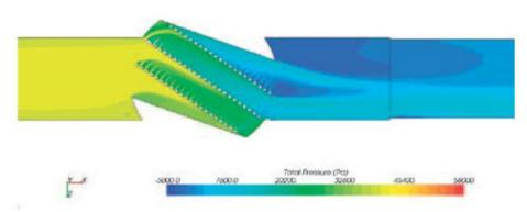
Compared to a standard ball valve, which is actually a two-stage valve, the multi-stage solutions ensures a very low pressure recovery factor, hence reducing flow velocity, ice formation and the risk of cavitation. The pressure energy is smoothly dissipated through the stages.
