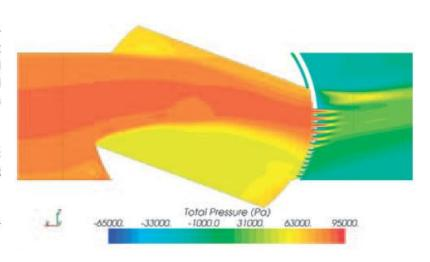
DAFRAM developed a proprietary calculation software for valve sizing and valve behaviour prediction; this special tool is based on DAFRAM CFD calculation data and on the mathematical model validation obtained through intensive bench testing sessions that allowed a refined setting of the virtual model for each trim configuration.
